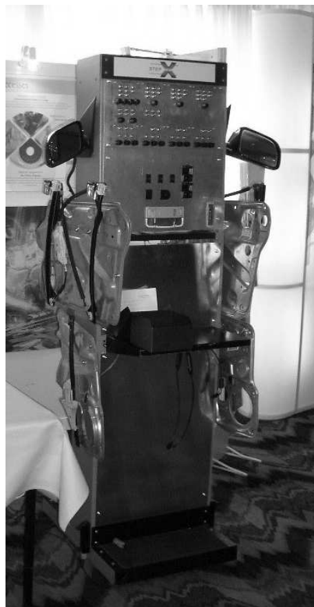
Figure 2 STEP-X demonstrator of a comfort systems (4 doors)
